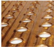
**Marlo "M" Fin** - designed with a less pronounced wave than a Turbex fin, this V-waffle fin offers a balance between high heat transfer efficiency and low air pressure drop.
