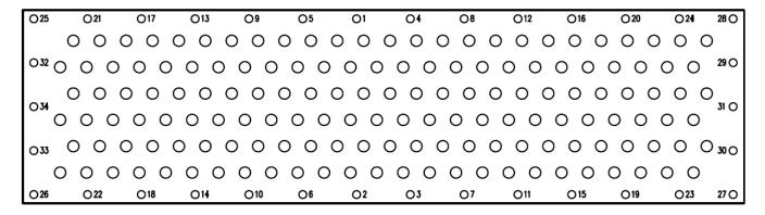
Figure 2 - Typical Bolt Sequence
